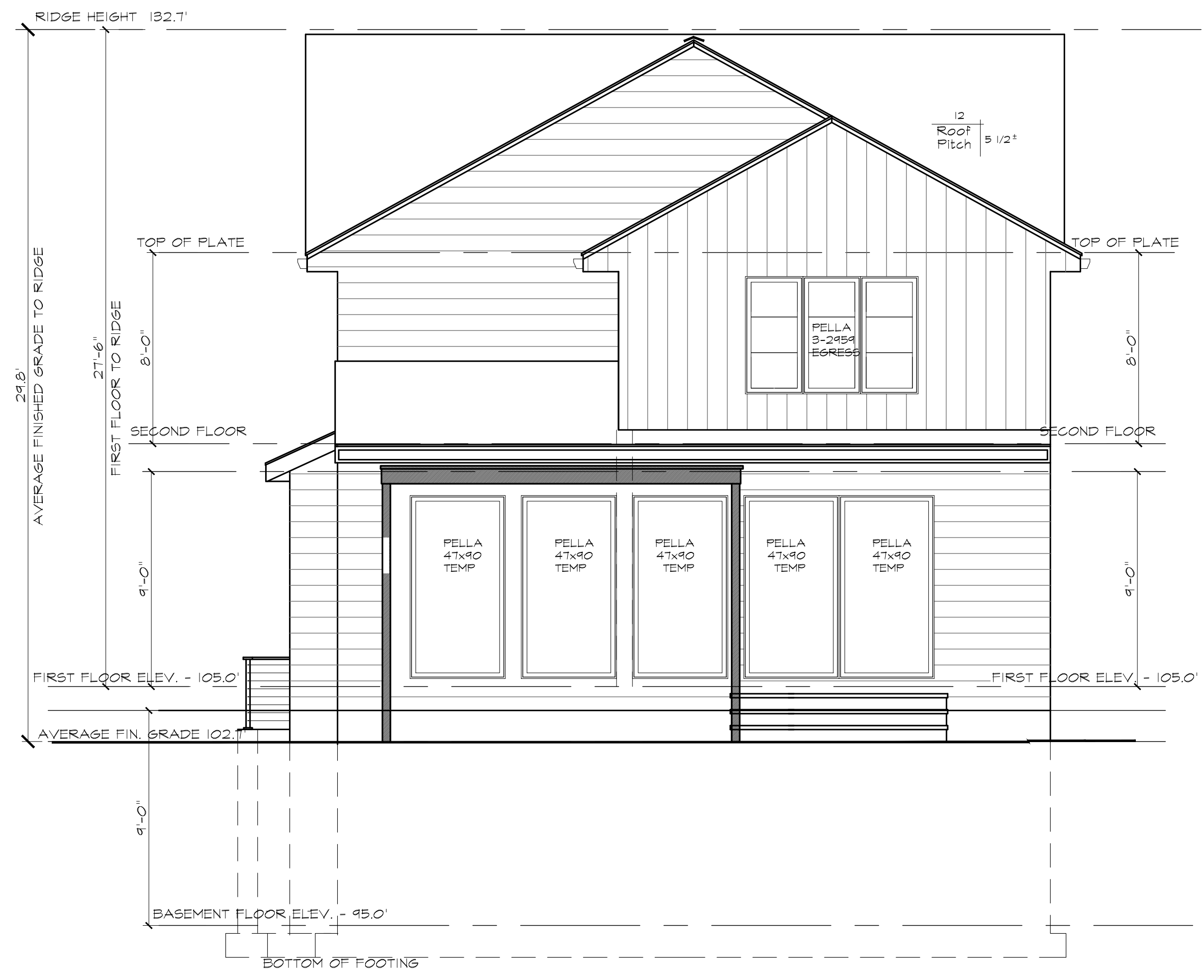
REAR (SOUTH) ELEVATION SCALE: 1/4" = 1'-0"
